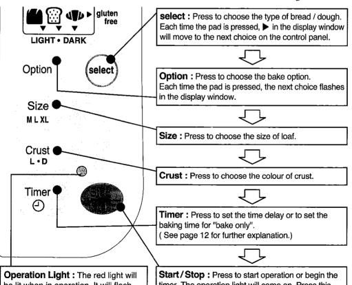
be lit when in operation. It will flash when the bread baking or the dough making is completed. It will also flash in a different frequency when operated in abnormal conditions.
